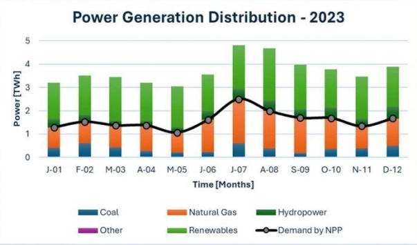
Figure 1. Monthly distribution of the total Power Generation during the year 2023. The curve indicates the power that SMRs could replace.
